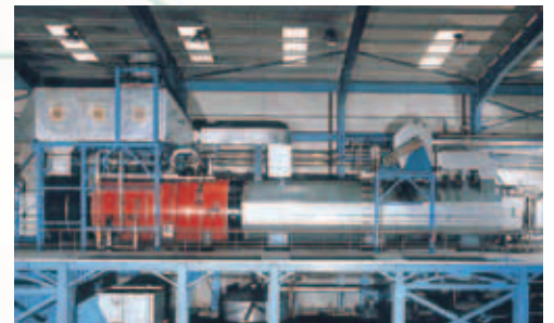
Rendering industry • Heat recovery oxidiser for steam production
