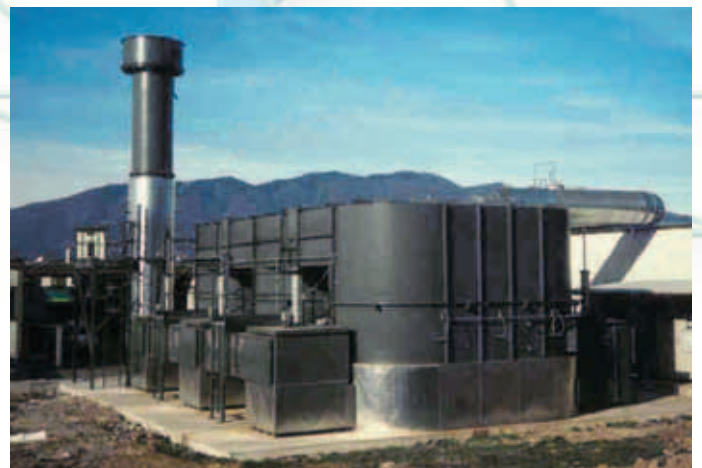
Rotogravure printing on flexible support • 40,000 Nm 3 /h
