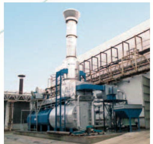
Rendering industry Thermal fluid heat recovery oxidiser
